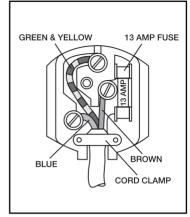
13 amp ASTA approved (BS 1362) fuse must be used. Should the plug need to be replaced for any reason. The wires in the mains lead are coloured in accordance with the following code:
